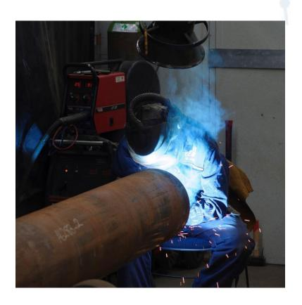
Where flexible arm fume extraction is used, the position of the extraction hood is crucial! If too far away, it has no benefit; it typically needs to be placed within 30cm of the welding source although this range may be much shorter. And so it is important that the system's capture range is identified during commissioning and further routine testing of the LEV system.
