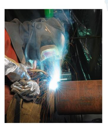
The welder is being exposed to welding fume and gases, which are not being properly controlled.
