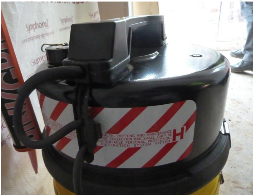
Picture illustrates H class vacuum for use with on-tool extraction and for cleaning up.
