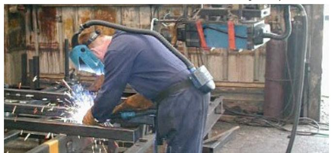
Welding fume exposure can be minimised by the use of local exhaust ventilation (LEV), including on-tool extraction. The Welding institute and others have demonstrated that effective control using LEV does not have any impact on the quality of the weld and protects workers from hazardous fumes.
